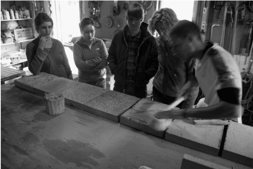
2. Experimenting with surface treatments on the fly ash concrete samples in the wood shop. Remote Studio base, June 1, 2010. (Photo by Chris Taylor.)
